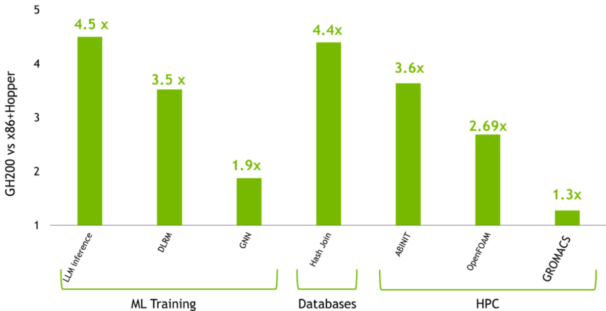
Figure 12. Performance Simulations for GH200 with HBM3 vs x86+Hopper for end-user applications. Datasets and details described in the individual application section below.
